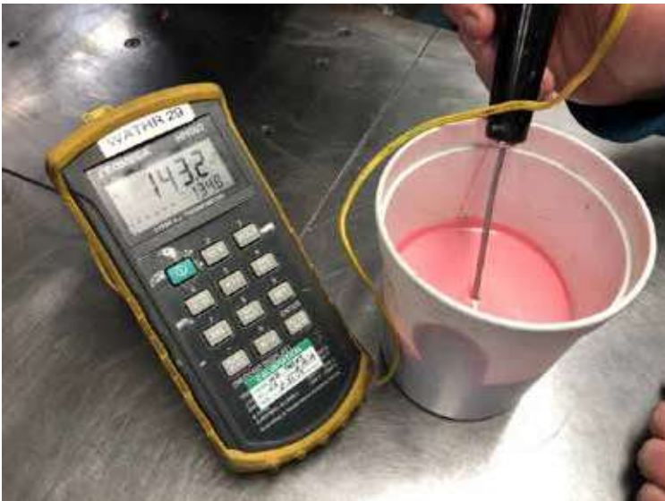
Example 1: Wax temperature measurement at the nozzle tip. First purge the wax in the nozzle then fill at least ½ the volume of a quart cup container. Immediately insert a small tip temperature measuring device that have been calibrated and allow to reach the maximum temperature.
