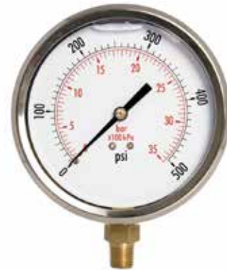
Example 2: A certified gauge can be acquired from industrial suppliers or gauge manufacturers. These are typically oil-filled and chosen knowing the pressure typically measured and assuring the gauge reads this pressure near the mid-point of its display.
